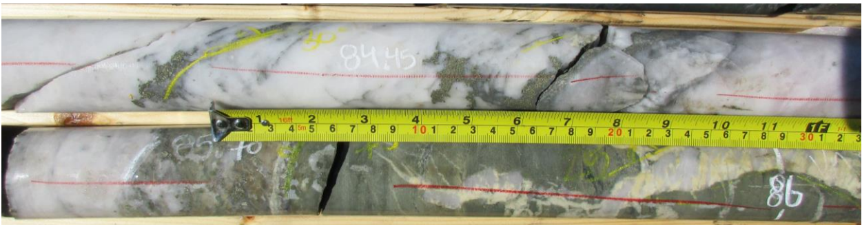
Figure 2: Hole 4 (ACP-R-21004) 84.25 metres to 86.05 metres; Multi-stage quartz-carbonate vein showing boudinage texture of early vein and later massive quartz-carb vein with sulphides.
