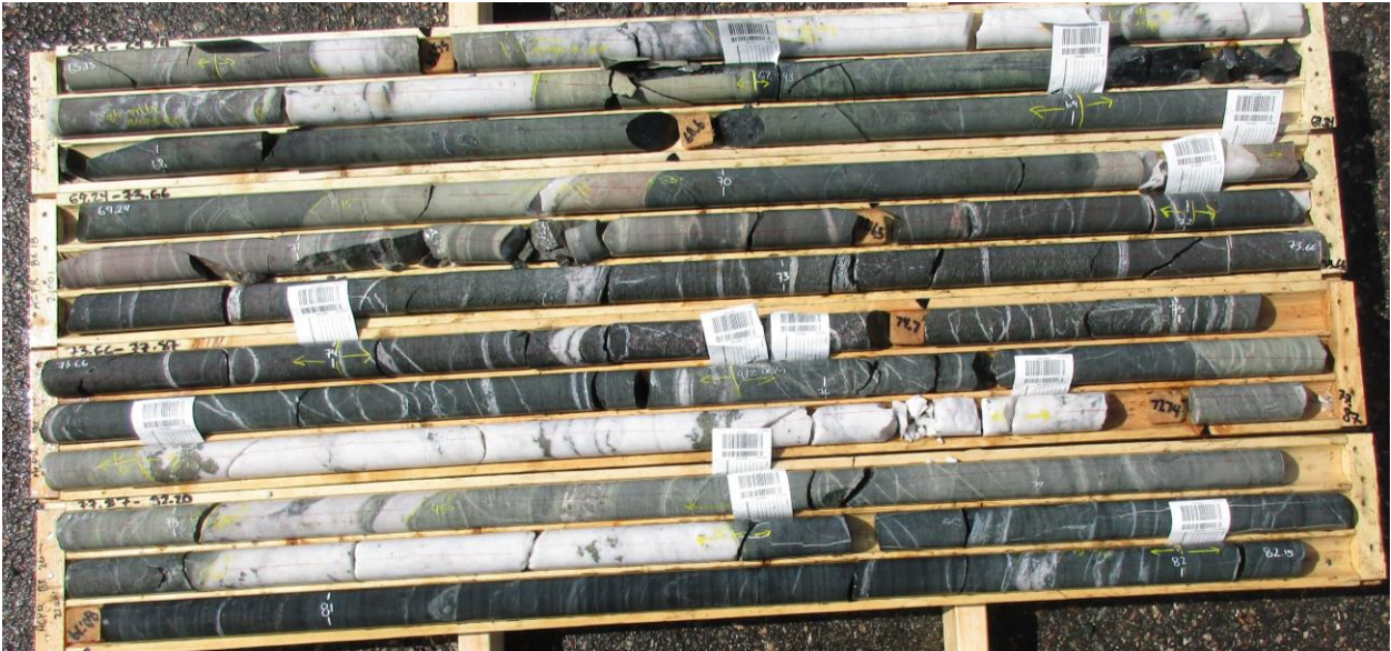
Figure 1: Hole 1 (ACP-R-21001) at Rickard Project, 65.13 meters to 82.15 meters (core boxes are 5 feet wide) showing two of three quartz carbonate veins intersected in hole 1.
