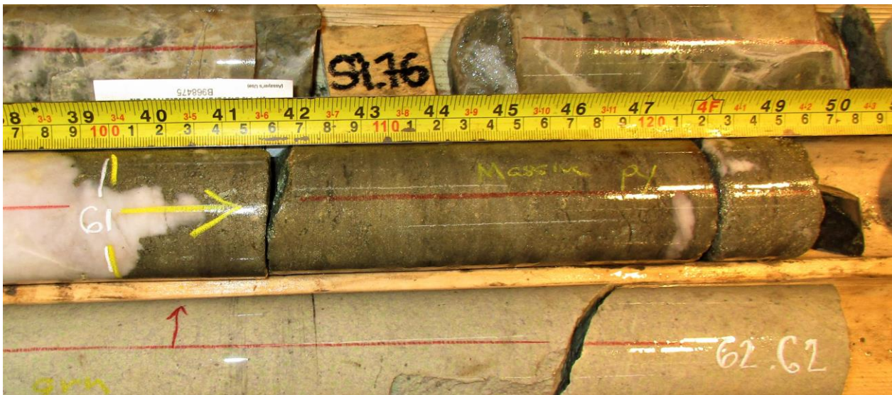
Figure 2: Hole 12 (ACP-R-210012) 60.89 metres – 61.25 metres showing partial section of a massive sulphide intersection contained within the center of a larger quartz-carbonate vein.
