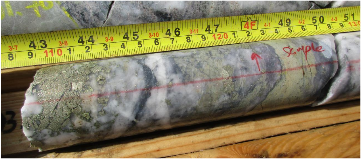
Figure 1: Hole 9 (ACP-R-21009) 103.09 to 103.28 metres showing smoky quartz vein section within larger quartz carbonate vein interval with abundant sulphide content and strongly altered clasts.
