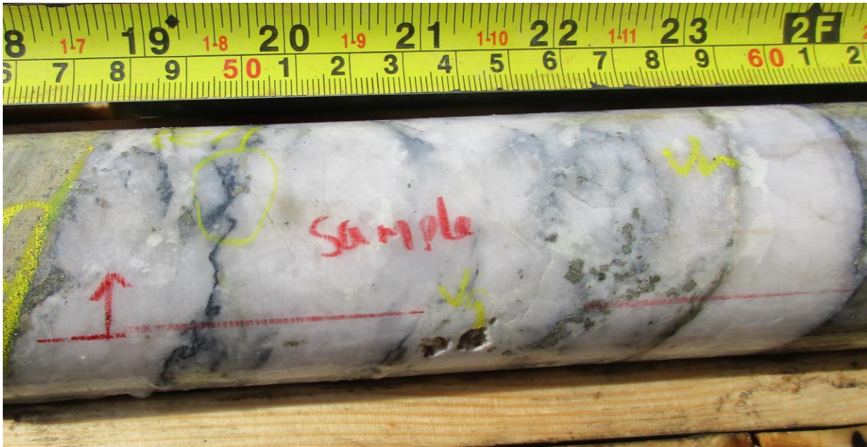
Figure 3: ACP-R-21009 – Quartz-carb veins with Stylolitic band showing molybdenite, with possibly graphite and telluride minerals, similar-to those seen in the Macassa Mine 70km to the south.
