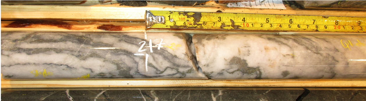
Figure 3: Hole 17 (ACP-R-210017) at 217.0 metres showing quartz-carbonate vein with wavy stylolitic bands of pyrite molybdenite chalcopyrite and blebby chalcopyrite and pyrite with sericitic lenses.
