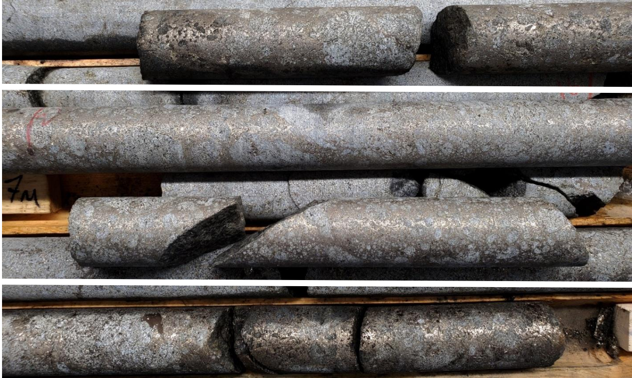
Figure 2: Drill hole VW-23-04 drill core showing net texture and sulfide-matrix breccia textures from 14 to 14.5 (top) from 20.5 to 21.5 (middle) and from 19.5 to 20 (bottom).
