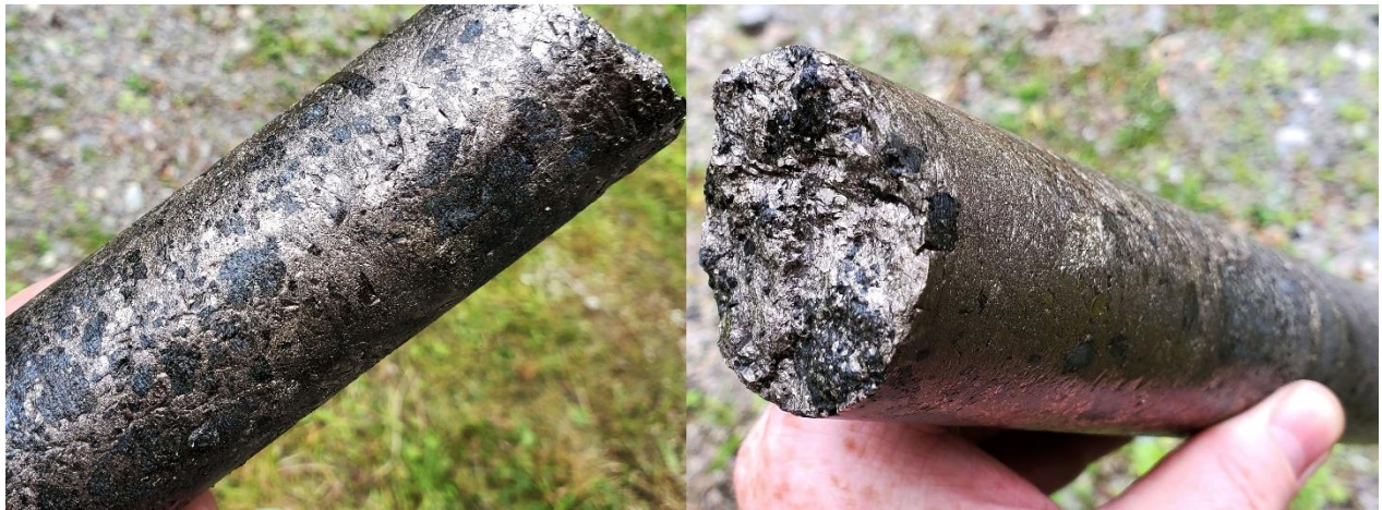
Figure 1: Core photo from VW-23-04 at 19.8 metres down hole (left) and 20.2 metres (right) showing net-texture, sulfide-matrix to massive texture.
