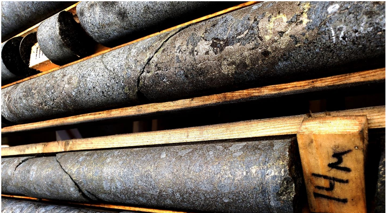
Figure 4: Hole VW-23-05 from 12 and 14 metres downhole showing net-textured and blebby massive sulphides with higher concentration of visible copper (chalcopyrite) with visually identified nickel sulfide and pyrrhotite.
