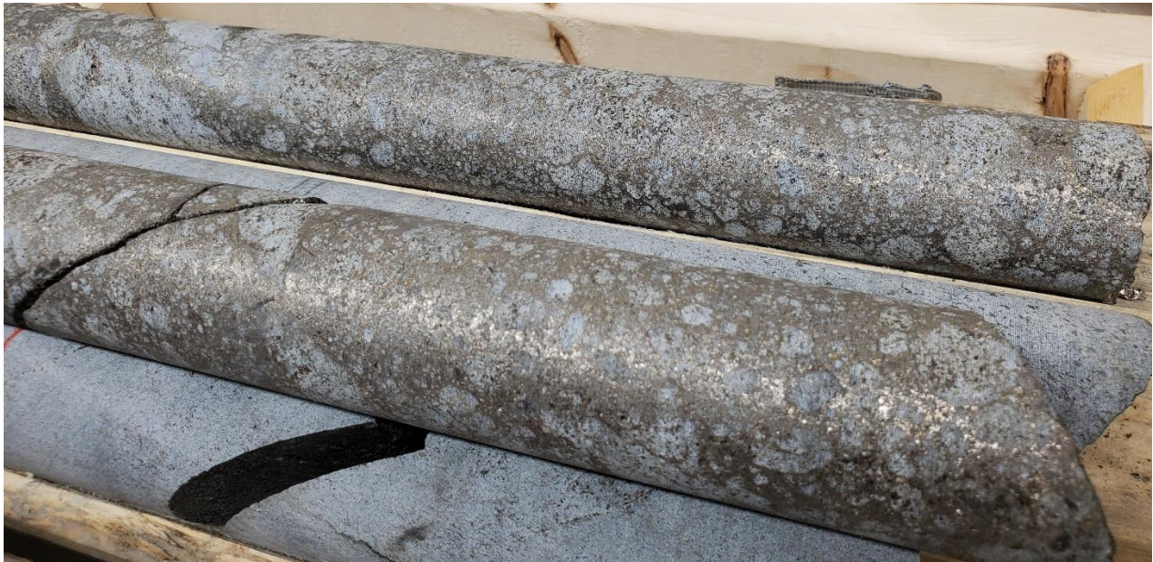
Figure 2: Core photo from VW-23-04 (dry core) at 21 to 22 metres down hole showing net-texture, sulfide-matrix texture. Assays from VW-23-04 are pending.
